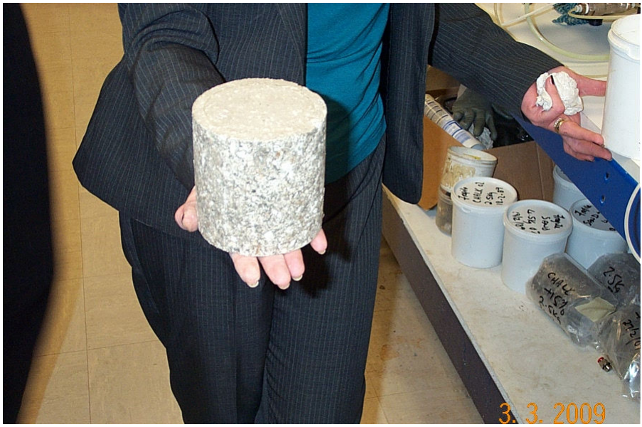
Figure 3. Compacted chalky sub-soil sample with cement inclusion
