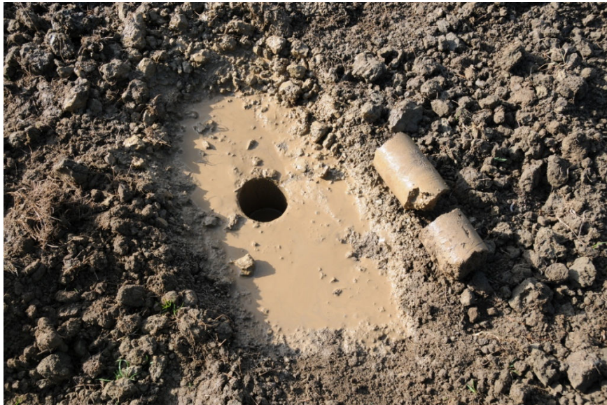
Figure 14. Bridge Farm - after core removed
