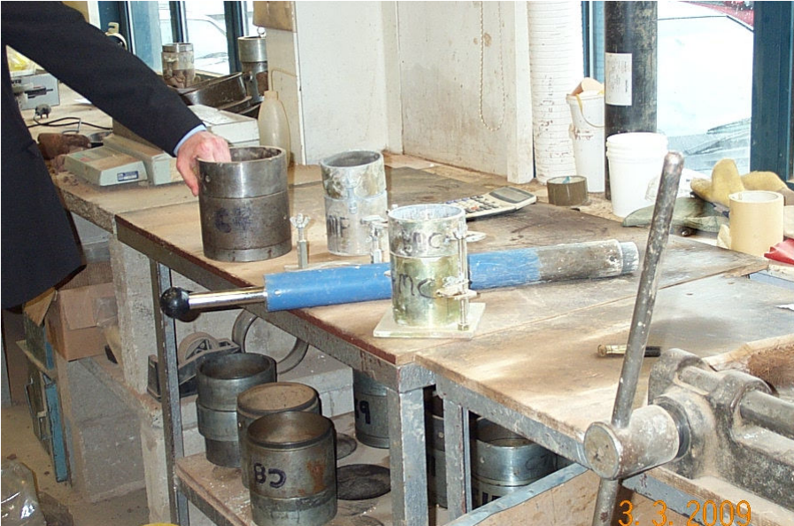
Figure 2. Sub-soil sample moulds and compacting instrument – GeoTest laboratory
