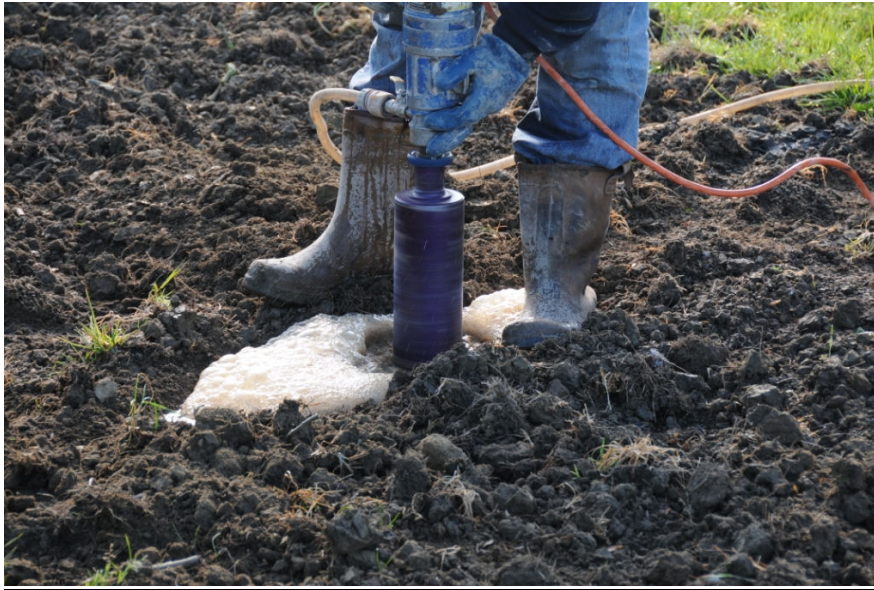
Figure 13. Bridge Farm - coring the cow track
