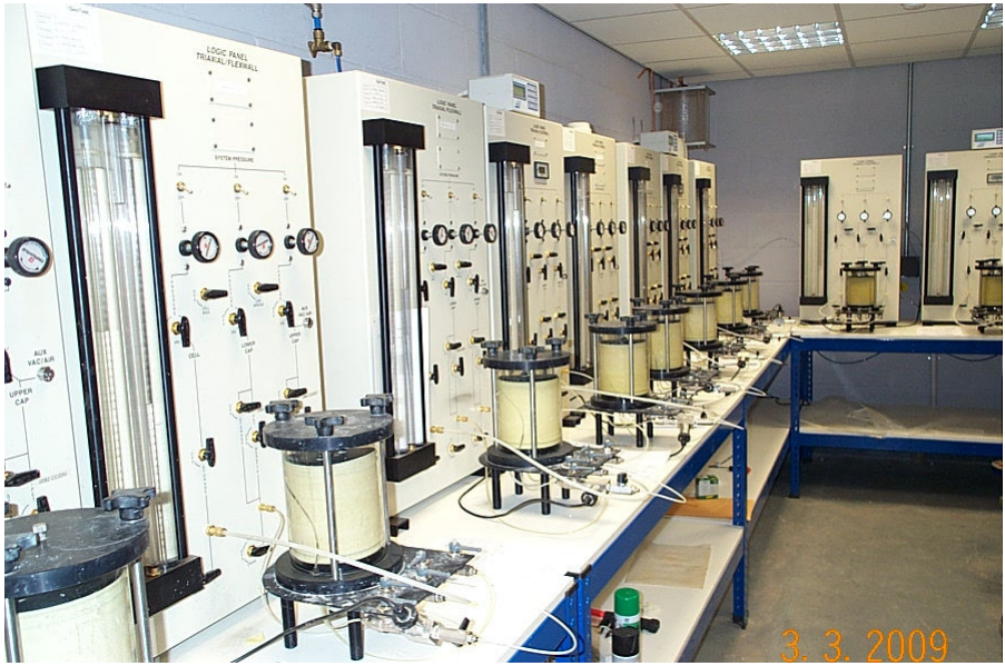
Figure 4. Sub-soil samples - Permeability testing at GeoTest laboratory
